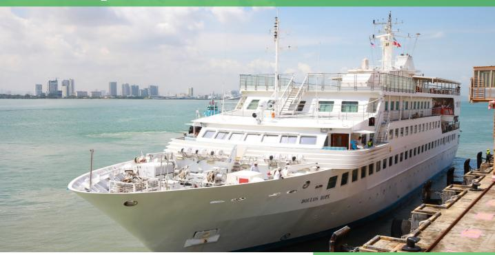
The are delighted to introduce OM's new ship, *Doulos Hope*. With five decks and a capacity of around 140 crew members, *Doulos Hope* is a smaller vessel with less draft than her sister ship, *Logos Hope*, enabling her to operate in shallower waters and travel to new regions. The ship will be based in Southeast Asia and stay in ports for extended periods to enable greater cultural engagement.
